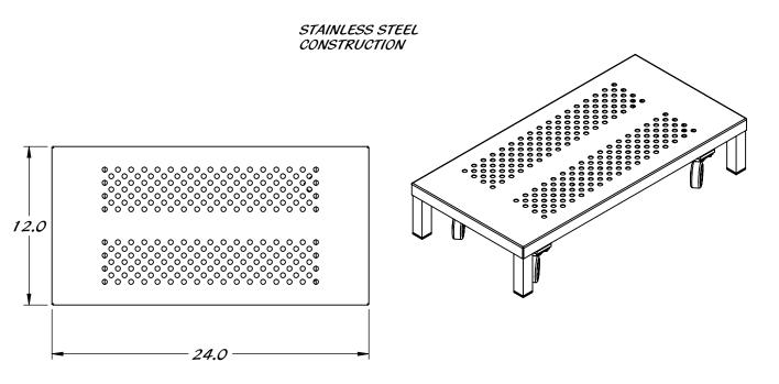
STEP STOOL CAN BE ROLLED INTO LOCATION. WHEN WEIGHT IS APPLIED, STEP STOOL WILL NO LONGER ROLL.
